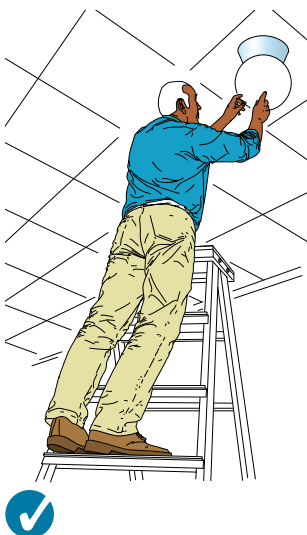
Figure 12 Correct - three clear steps. Don't work any higher up this type of stepladder
