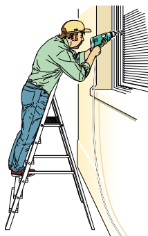
Figure 2b Correct - steps facing work activity
