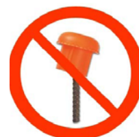
Figure 2: Typical example of an incorrectly fitted rebar-cap
